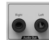
The KB37 features a stereo signal path that is also buffered by an output stage. Even when you're using a mono setup within your module patches it's not a bad idea to make a two-channel connection to your mixer. As long as you use the *Left / Mono In* jack only on the front panel, the signal is sent to both outputs. This way you can switch between mono and stereo output quickly by just inserting a patch cable.
