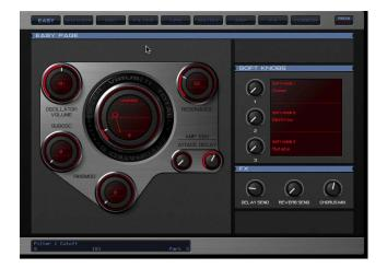
The large controller in the centre of the page is the filter control – turn the dial to change the Cutoff, or try moving the little red square to sweep Cutoff and Resonance simultaneously. The filter type can be adjusted by clicking on 'Lowpass' and moving the mouse vertically.
