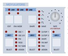
LFOs (Low Frequency Oscillators) are often used to add some cyclic movement to otherwise static sounds. There are three LFOs in your Virus, and each one has a different assortment of preset destinations it can modulate directly.
