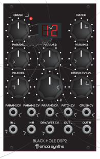
The encoder has several features. Rotate the encoder to select one of 24 effects. Push the encoder promptly to confirm the selection and activate the effect. Push and hold the encoder to save (a display will indicate SA) all parameter settings with the effect!
