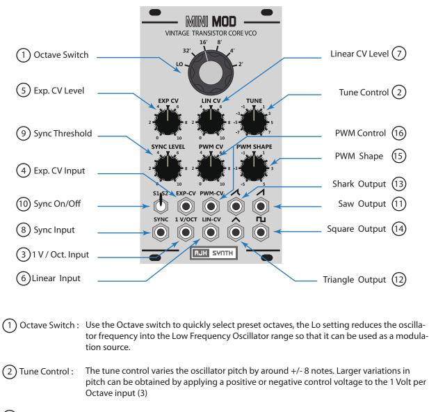
(3) 1 V/Oct. Input: This is the 1 Volt per Octave control voltage input. Applying a positive voltage to this input raises oscillator pitch at the rate of exactly one octave for each volt applied, and a negative voltage will reduce the pitch by exactly one octave per volt. The acceptable input range is +/- 7 Volts. A limitation of the vintage oscillator core design means that tracking may not follow the 1V/Oct law above 10KHz
