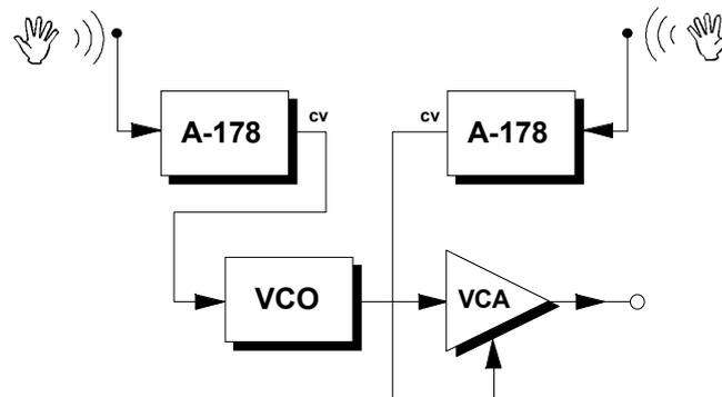
fig. 1: A standard theremin, using two A-178 modules
