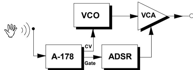
fig. 3: User example for the gate function
