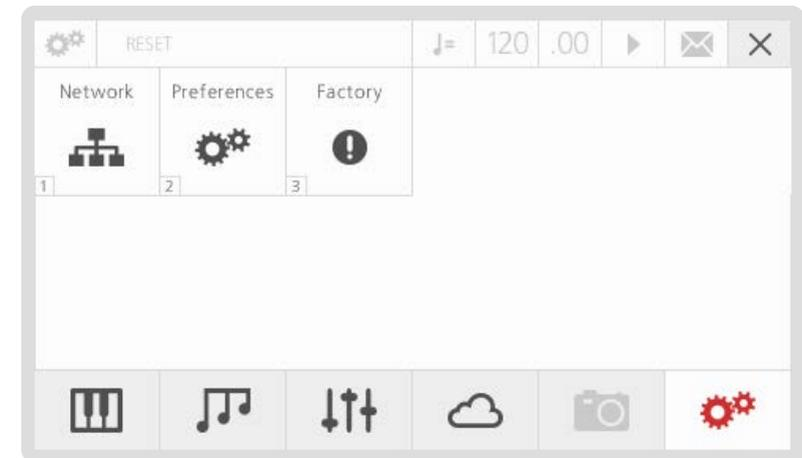
1. **Network:** this option resets all Network settings and it is very useful anytime you connect the 008 to a different router or in a different network configuration
