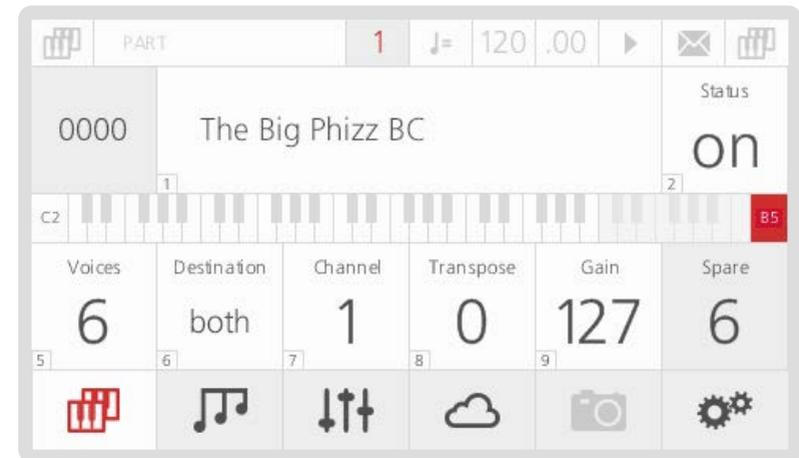
1. **Patch Name/Number:** these two boxes show slot number and name of the the patch which is currently used by the selected part. The Name box can be used to load patches in the same way that regular patches are loaded (see chapter 1).
