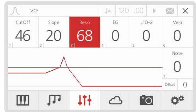
Modal 002 provides two separate classic 4-stage contour generators (i.e. envelopes), one for the filter (VCF-EG), one for the amplifier (VCA-EG): the former modulates the filter cutoff frequency, if a value different from zero is set for the filter EG parameter (see 'Filter' section - previously in this same chapter); the latter modulates the amplifier volume, if a value different from zero is set for its own Amount parameter.
