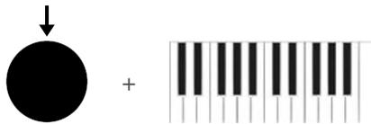
Holding down a sequence encoder that is part of a note row and playing a note on the keyboard inserts the played note into the held down step.
