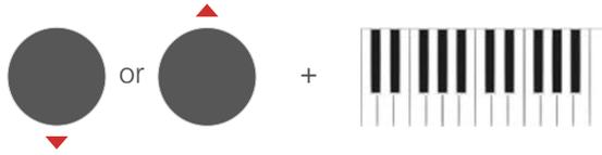
Holding down the Up/Down button next to the Note or empty row you want to edit you can input notes using the keyboard. The first note pressed will be inserted into the Sequencer start step. After each key is pressed the next key will be inserted into the next step, which allows you to quickly play a sequence into a note row. This shortcut can also be used on CC rows, where the keyboard can be used to assign values.
