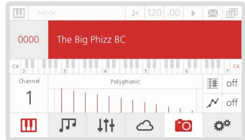
When Snapshot is enabled or disabled the user is kept on the current page. A useful example of this functionality is when a user has changed some filter settings on the VCF page but wants to know what the original filter settings were. Pressing the snapshot button will show the saved settings, then pressing again will show the current settings.
