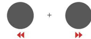
Pressing the Left and Right buttons down at the same time will turn the Arpeggiator status on and off. It is also a quick way to get to the Arpeggiator screen.
