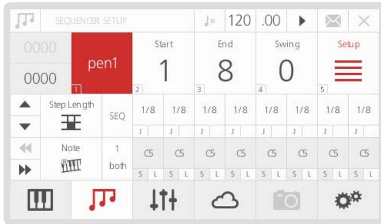
**Values:** Each row contains a set of 8 steps and each step has its largest part showing its current value (e.g. note number, CC value, step length, velocity and gate length). These values can be edited by turning the front panel push-dials and/or by using screen controls.
