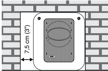
into the right end of the recess with the driver side facing the room. This leaves sufficient 7,5 centimeters (3") of free space on the reflex port side. The height and depth of the recess should not be any bigger than those needed to fit the subwoofer flush with the wall surface.
