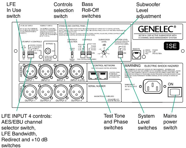
Connect the signal cables for the main loudspeakers to the male "AES/EBU OUTPUT" connectors on the subwoofer. Each of these connectors carries a high-pass filtered version of the signal(s) received by the input connector marked with the same number. The default filtering frequency is 85 Hz. The filtering frequency cannot be changed with the controls available in the stand-alone mode. This feature is only available when the subwoofer is controlled by the GLM.SE™ software.
