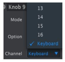
The "Keyboard" option allows you to change the MIDI channel of this control when you change the MIDI channel setting of the keyboard.
