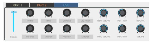
Encoders 6-8 and 14-16 work the same as they do for Parts 1 and 2: one parameter per encoder. So click on their labels and select the parameter you want to control.
