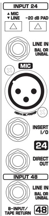
Fig. 7.8: A and B-channel input section
