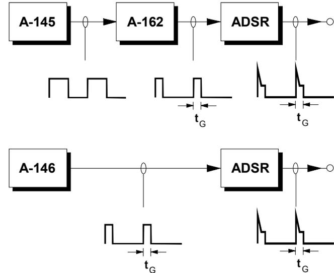
**Fig. 3:** Producing gate pulses of variable duration
