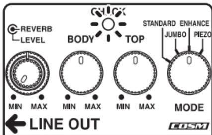
1. When you have made the necessary connections (p. 6–p. 11), set the knobs as shown in the illustration.
