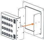
**Flush mounting in a wall** Use the mounting frame AH11504 in the orientation shown below. Align the threaded inserts on the sides of the DT164-W with the frame, and secure the unit in place with the 6x M4 6mm T20 screws provided. Connect the power and Cat5 cable/s, then fix the assembly to the wall using appropriate fixings or screws for the type of wall.
