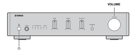
1 Press the 🖰 (power) button on the front panel to turn on the unit.
