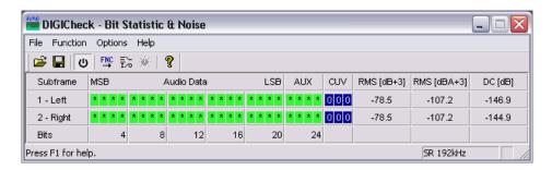
The reason for this behaviour is the noise shaping technology of the analog to digital converters. They move all noise and distortion to the in-audible higher frequency range, above 45 kHz. Therefore the noise is slightly increased in the ultrasound area. High-frequent noise has a high energy. Add the quadrupled bandwidth, and a wideband measurement will show a significant drop in SNR, while the human ear will notice absolutely no change in the audible noise floor.
