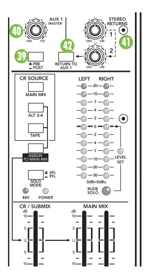
So, the original "dry" signals go from the channels to the main mix and the affected "wet" signals go from the stereo return to the main mix, and once mixed together, the dry and wet signals combine to create a glorious sound. So, armed with this knowledge, let's visit the Auxiliary World:
