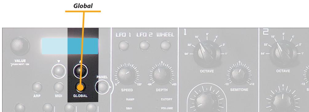
The Global function summarizes all general controls of the instruments, not related to a specific sound or program. The list of controls and their meaning is as it follows:
