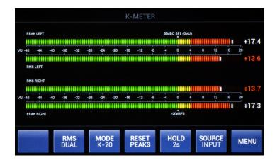
K-metering system build in the Mastering Limiter supports **K-12**, **K-14 and K-20** standards. It helps you calibrate your studio monitoring levels and produce more consistent music content, while still maintaining high dynamic range.
