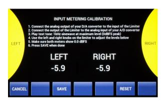
The Mastering Limiter is prepared to work straight form the box. In most cases the metering will be accurate and the limiter will behave perfectly. However if you would like to calibrate the internal metering to match your AD/DA readouts, please perform simple calibration procedure. Make sure you always calibrate input metering first and then output.
