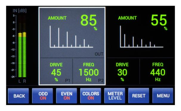
Use the ON/OFF buttons on the bottom of the screen to enable or disable one or both of the harmonic generators (colors). Press **RESET** to set the generators settings to their default values. Use **METER** to switch to GR metering.
