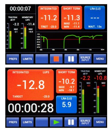
There are two types of layouts to choose from in **PREFS** window. You can also change integration time for LRA (20 or 60 secs of collecting samples before LRA value is given), change LUFS and LKFS units and set the timeout for warnings. If INFINITE WARNING HOLD is ON then every value that is above or under set limits will stay red until the end of the measurement.
