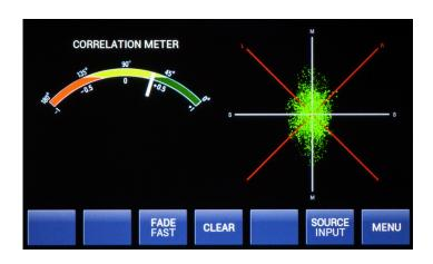
Pressing **FADE** button will toggle between different fade timeouts. **CLEAR** will reset the correlation graph.
