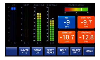
By tapping on different parts of the screen you can scroll thru all available measurements. The Limiter will remember your choices. As there are three CUSTOM sets available you can use them for different jobs, for example: mixing, TV mastering, audio stream mastering.
