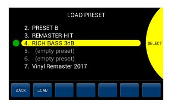
Loading presets is very simple too. Just Press **LOAD** in the Main Menu, choose the preset and hit LOAD in the LOAD PRESET window. The Mastering Limiter will recall all the settings and activate the ENGAGE. Press BACK or scroll thru other presets to find the one that suits your needs.
