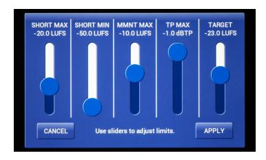
**LIMITS** window allows you to set targets for the analysis. If any of the values goes above or under this limits it will turn red. You can set desired range for short term loudness, maximum momentary loudness, maximum TruePeak level (the limiter uses 4x oversampling to calculate level) and most importantly - the target for Integrated Loudness
