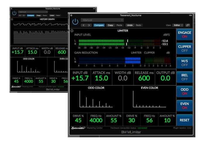
connection. The unit appear as a HID device and can be managed via Bettermaker Mastering Limiter Plugin.
