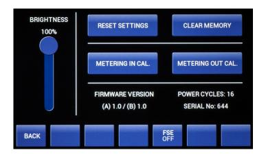
This screen allows you to adjust the **BRIGHTNESS** of the screen (touch and drag the virtual slider on the screen), check the firmware version of your unit, see the number of power cycles (how many times the unit was turned off and on), but also to **CLEAR** presets memory and perform the **METERING CALIBRATION** procedure (it has to be done only
