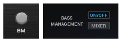
Mirrors the Control Panel Bass Management On/Off Switch. Useful for checking between having the LFE channel play all low-frequency contents of the mix or only its designated signal.
