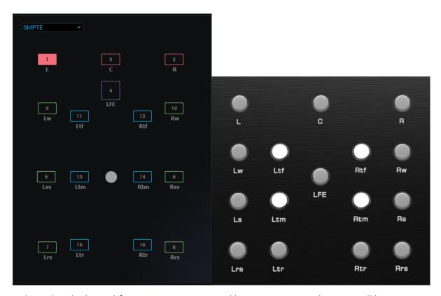
Selected multichannel formats are represented here. Buttons on the MRC will become inactive when their respective speakers are not part of the selected format.
