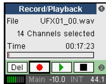
**Transport Bar.** Turning encoder 2 moves the cursor over *Del* (Delete), *Record*, *Play/Pause* and *Stop*. The selected function is initiated by pressing encoder 2. During playback the buttons *Del* / *Record* will change to *Previous File* / *Next File*.
