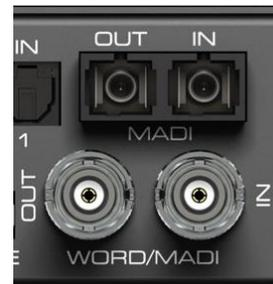
Selecting *Single Speed* in the Settings dialog causes the output signal to always stay within the range of 32 kHz to 48 kHz. So at 96 kHz and 192 kHz sample rate, the output word clock is 48 kHz.
