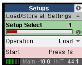
The Fireface UFX+ can store and load its current state in 6 different memory slots, called Setups. With this, the Fireface UFX+ can be used stand-alone after setting it up accordingly, replacing lots of dedicated devices (see chapter 24).
