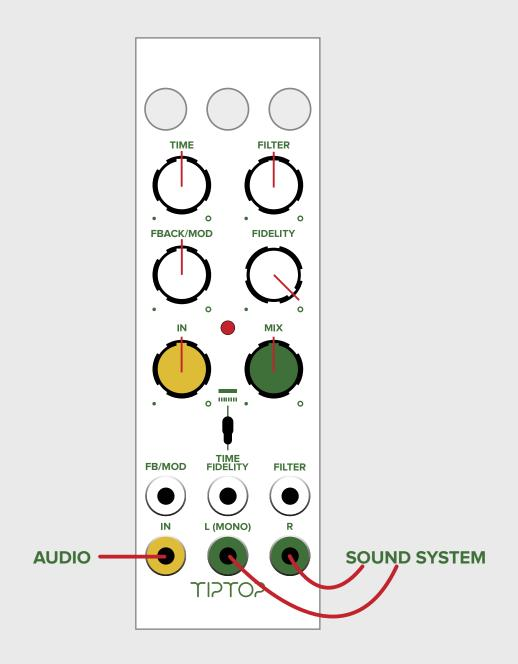
Set the Fidelity to max (CW), turn on power, patch audio into the In jack, patch the left and right output to your sound system. Make sure to patch both left and right so you get the full joy of stereo. Set the following knobs to the center: MIX, IN, TIME, FILTER, FEEDBACK/MOD.
