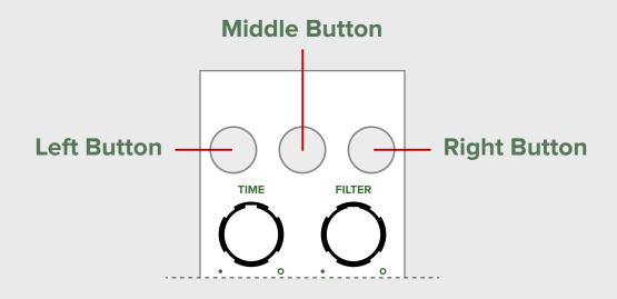
**Time knob** - controls the decay time of Reverbs, the Delay time or the rate of Modulation LFOs
