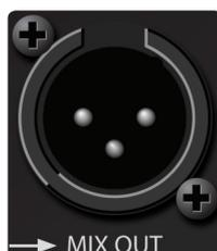
**Mix Out.** A balanced Mix output is provided on an XLR-M connector. The Mix Out connection is used to send signals connected to the inputs of your loudspeaker to other StudioLive-series loudspeakers. The Mix output signal is the same as the signal sent to the loudspeaker's internal amplifier, and it may be derived from the microphone input, the line input, or a mix of both.
