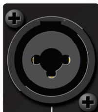
**Line Input.** This is a balanced XLR / 1/4" TRS combo connection for line-level input. Use the Line input to connect the loudspeaker to a StudioLive digital mixer or other mixing console, either directly or through the Line in/out connectors on a StudioLive S18sAI subwoofer. The Line input will accept a signal level of up to +24 dBu before clipping.
