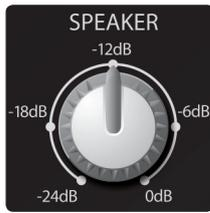
**Speaker Level.** This control attenuates the output level of your StudioLive full-range loudspeaker's internal amplifier. As with the Line Input level control, in most situations, you can set this knob fully clockwise to the 0 dB setting.
