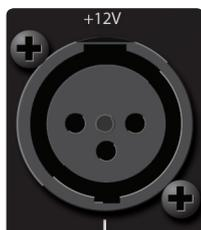
**Microphone Input.** Your AI-series full-range loudspeaker is equipped with a PreSonus XMAX™ microphone preamplifier for use with most microphone types. The XMAX solid-state preamplifier has a Class A input buffer, followed by a dual-servo gain stage. This arrangement results in ultra-low noise and wide gain control, allowing you to boost signals without increasing unwanted background noise.
