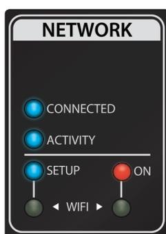
**Network Status and Controls.** These LEDs and controls provide information about network connectivity and allow you to configure your included wireless LAN adapter.
