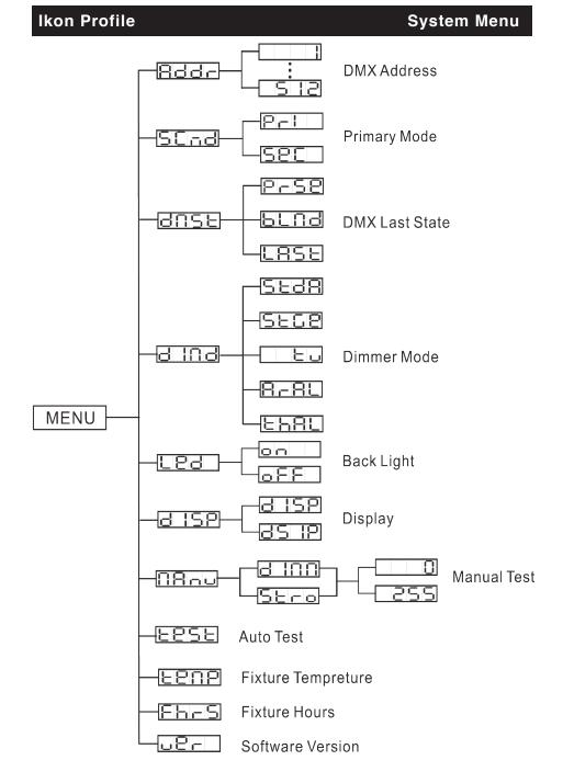
**On-Board System Menu.** The Ikon Profile comes with an easy to navigate system menu. This next section will detail the functions of each command in the system menu. **Please read the next section thoroughly!**
