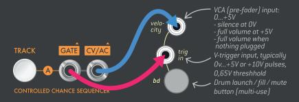
Every drum channel has a CV VCA controlled Velocity input, which defines the amplitude (volume) of the drum channel. When no plug is inserted into the velocity jack, the volume of that channel is maximum by default. Think of the Velocity input as either VCA to make accents for your drums, or as an envelope input to adjust the dynamics.
