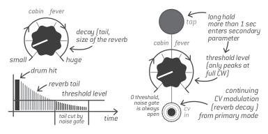
verb dry/wet amount and CABIN FEVER defines the reverb decay, as usually. However the secondary FEVER action defines the threshold of the noise gate — from zero (full CCW, sound always on) to max (full CW, only slight peaks). Default threshold value is 20%. This setting suits most of the drums. Noise gate's attack and decay are fixed and chosen experimentally to fit most musical styles.
