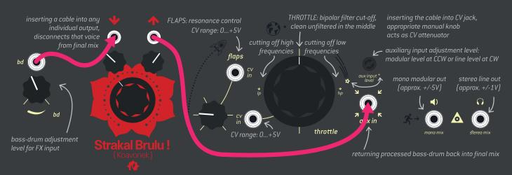
**FLAPS** is the resonance control of THROTTLE, and functions as a tone control for the output. Be aware: use FLAPS carefully: with higher values you may get a loud hi-frequency whistling sound that could damage your ears or PA. Filter controls THROTTLE and FLAPS influence only final outputs (and everything that is inserted into AUX IN), not separate outputs.
