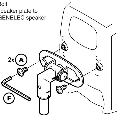
5.b Replace the bolt of the speaker plate
