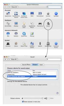
Figure 5-2: The Mac OS X sound preferences let you use the UltraLite-mk3 for general stereo audio input and output for your Mac.
