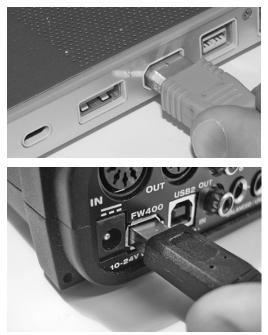
Figure 3-1: Connecting the UltraLite-mk3 to the computer via FireWire.
