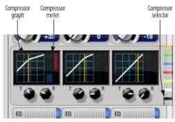
Figure 11-5: The Compressor controls.
