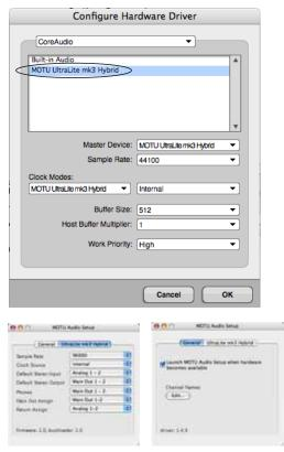
Figure 7-1: Choose Setup menu> Configure Audio System> Configure Hardware Driver to open the dialog shown above and access the UltraLite-mk3 Core Audio driver. To access the rest of the UltraLite-mk3 settings, open MOTU Audio Setup.
