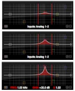
Figure 11-19: Type II EQ filter style.
