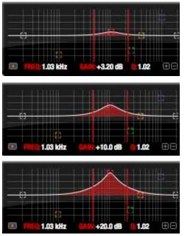
Figure 11-20: Type III EQ filter style.
