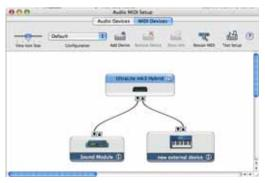
Figure 4-3: Connecting devices to the UltraLite-mk3. In this example, a controller keyboard is connected to the UltraLite-mk3's MIDI IN, and a sound module is connected to the UltraLite-mk3 MIDI OUT.
