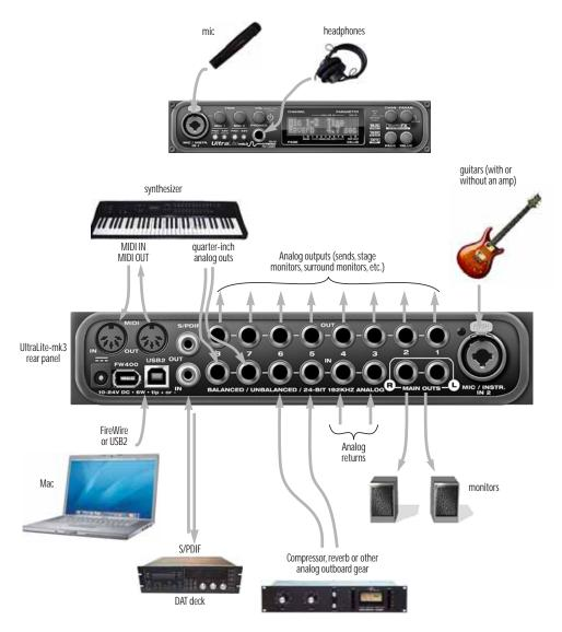
Figure 3-9: A typical UltraLite-mk3 studio setup.
