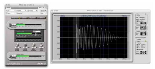
*Figure 11-39: Viewing transients in the Oscilloscope*
