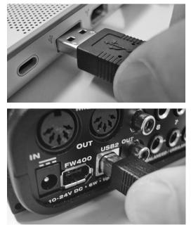
Figure 3-2: Connecting the UltraLite-mk3 to the computer via USB.
