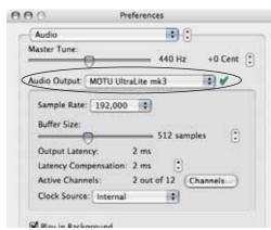
Figure 9-6: Enabling the UltraLite-mk3 in Reason.
