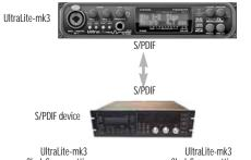
Clock Source setting = S/PDIF (when transferring from the other device to the UltraLite-mk3)
