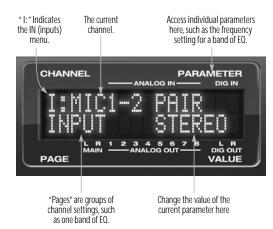
Figure 6-6: The IN (inputs) menu.
