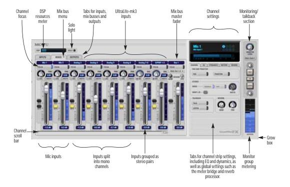
Figure 11-1: CueMix FX is a virtual mixer that gives you control over the UltraLite-mk3's on-board mixing features.
