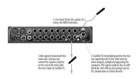
Figure 10-2: This diagram shows the signal flow when using CueMix FX no-latency monitoring. Notice that this method does not process the live input with plug-ins in your audio software. Instead, you can apply UltraLite-mk3 effects, such as the reverb, EQ and/or compression.
