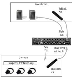
Figure 11-30: Typical hardware setup for Talkback and Listenback.
