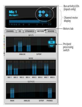
Figure 11-27: The Meters tab.
