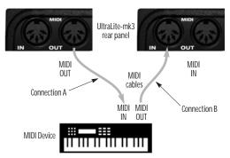
Figure 3-5: Connecting a MIDI device to the UltraLite-mk3.
