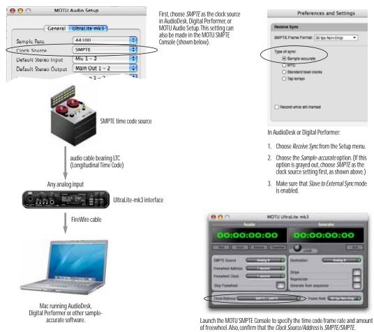
Figure 12-3: Connections for synchronizing the UltraLite-mk3 directly to SMPTE time code.
