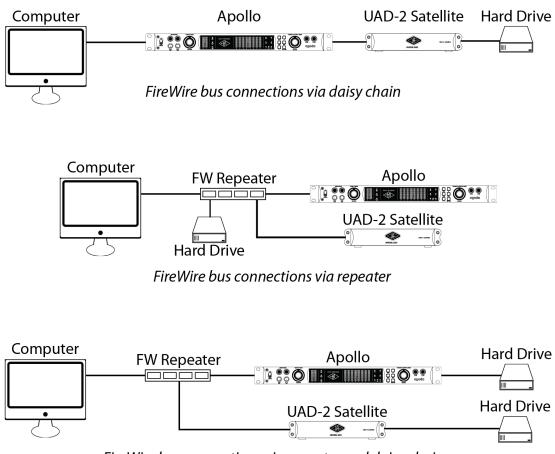
FireWire bus connections via repeater and daisy chain
