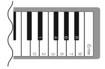
Axiom includes extended programming capabilities through secondary functions of the keys. The available parameters are listed along the top edge of the keyboard, and accessed by pressing the Edit button. The LCD screen shows the numerical value of the parameter being edited.
