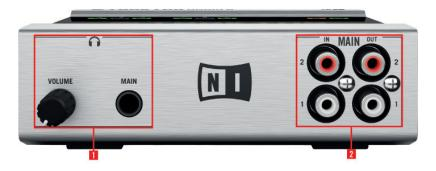
5.1 The front panel of the TRAKTOR AUDIO 6.
